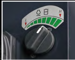
Engine speed (AUX flow) Control dial: 1050 - 2400 rpm (Attachment mode only)
