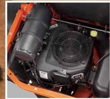
Z723/Z724/Z725 models (Powered by KOHLER® Command PRO engines) 22.5HP\*\*\*/23.5HP\*\*\*
